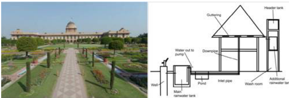
Fig. 4.5: Rainwater harvesting in Rashtrapati Bhawan.
